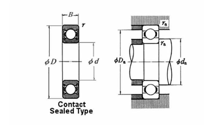
High quality Deep groove ball bearing with rubber contact seals from the world leader NSK, the worlds largest ball bearing manufacturer offering unparalelled quality. The unique & patented NSK DDU rubber seal features market leading technology, keeping contaminants and moisture out of the bearing while retaining the high class lubricant inside
